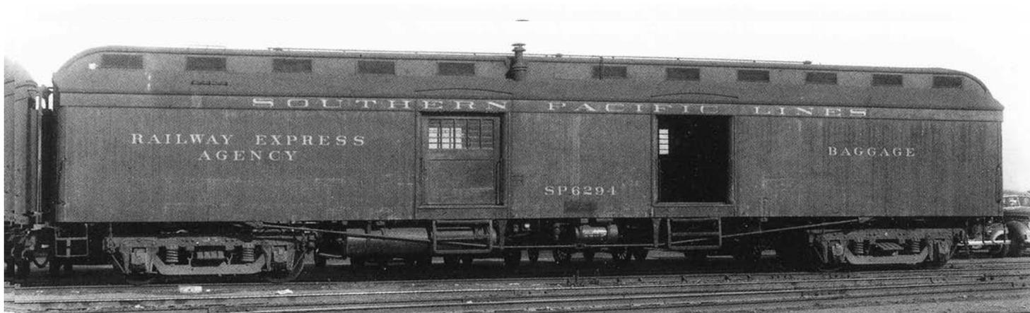
Nine cars built by AC&F in 1906 numbered SP 6284 - 6293, lettered Southern Pacific Lines. The lettering for these cars dates from 1940 with REA as the contract express company. With very slight modifications, this car can be modeled using Ultrascale kit #613.
